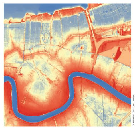
A LIDAR digital elevation model of a ten-mile-by-ten-mile area of New Orleans, captured in 2000, showing above-sea-level areas in red and lower areas in yellow and blue shades.
